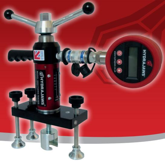
Connecting and disconnecting Gauges from the Tester body will eventually use up the spare oil capacity and will not allow the tester plunger to travel it's full stroke or give an accurate reading on the Gauge.
