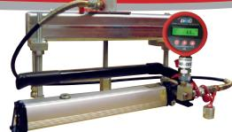
For use with hydraulic cylinder 125kN capacity or Model 2008 Tester
