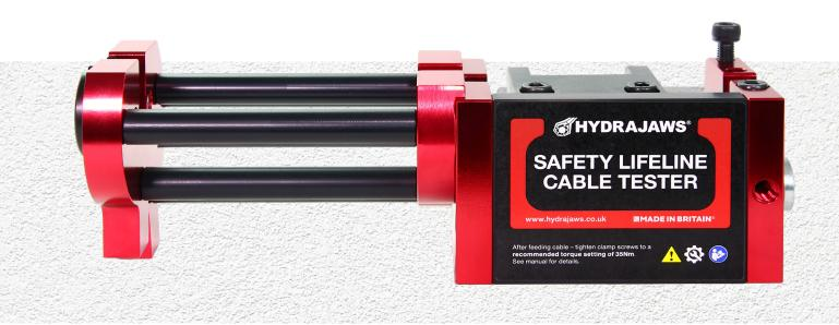
The **Hydrajaws Safety Lifeline Cable Tester KIT 1** (Frame Only) for operators who already own a M2000 Tester, enables engineers to validate the strength of swaged components of newly installed or existing engineered lifeline systems to ensure compliance with **BS7883** up to a maximum tensile load of **25kN**.
