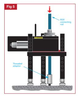
Connect the M20 connecting rod to fixing using the appropriate threaded adaptor (fig 6).
