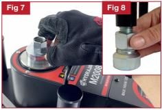
Adjust the 3 legs to an appropriate height, take up any initial slack using the threaded pull rod so that the fixing under test remains connected with no movement between the connecting rod nut and the top of the tester.
