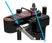
If after a test, the operating nut has been fully unwound and the top piston remains tight, untighten the adjustable nut with the ratchet spanner
