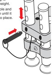
Fine adjustment can be made by unscrewing the feet by no more than approximately 10mm.
