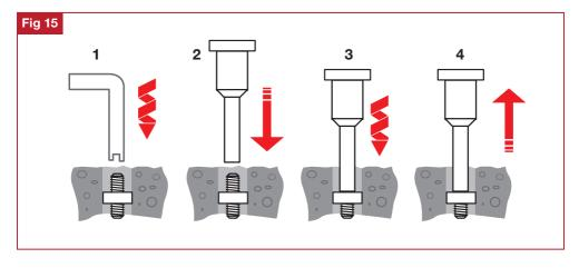
Remove the locking adaptor if fitted (see Section 1 General testing procedure). Adjust the length of the bridge legs and the height of the button adaptor/nut so that the adaptor can pass through the hole in the bridge and engage it in the pulling jaw of the tester (fig 16).
