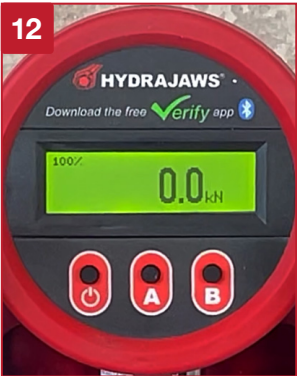
Turn the Gauge on and ensure it shows 0kN.
