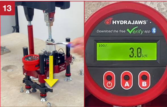
Preload the tester to a minimum of 3kN, and do not exceed 3.5kN.
