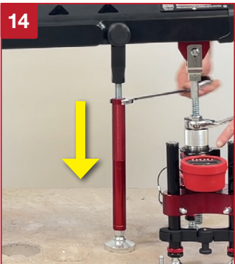
Wind Leg down to release the Preload, down to 0kN.
