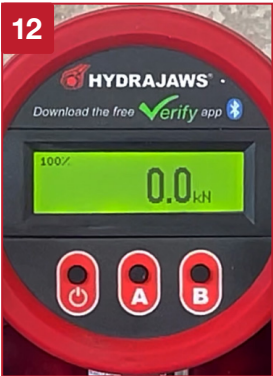
Turn the Gauge on, set to 0kN if required.
