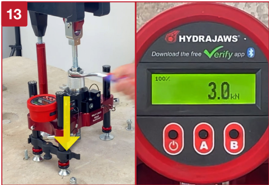
Preload the tester to a minimum of 3kN, and do not exceed 3.5kN.
